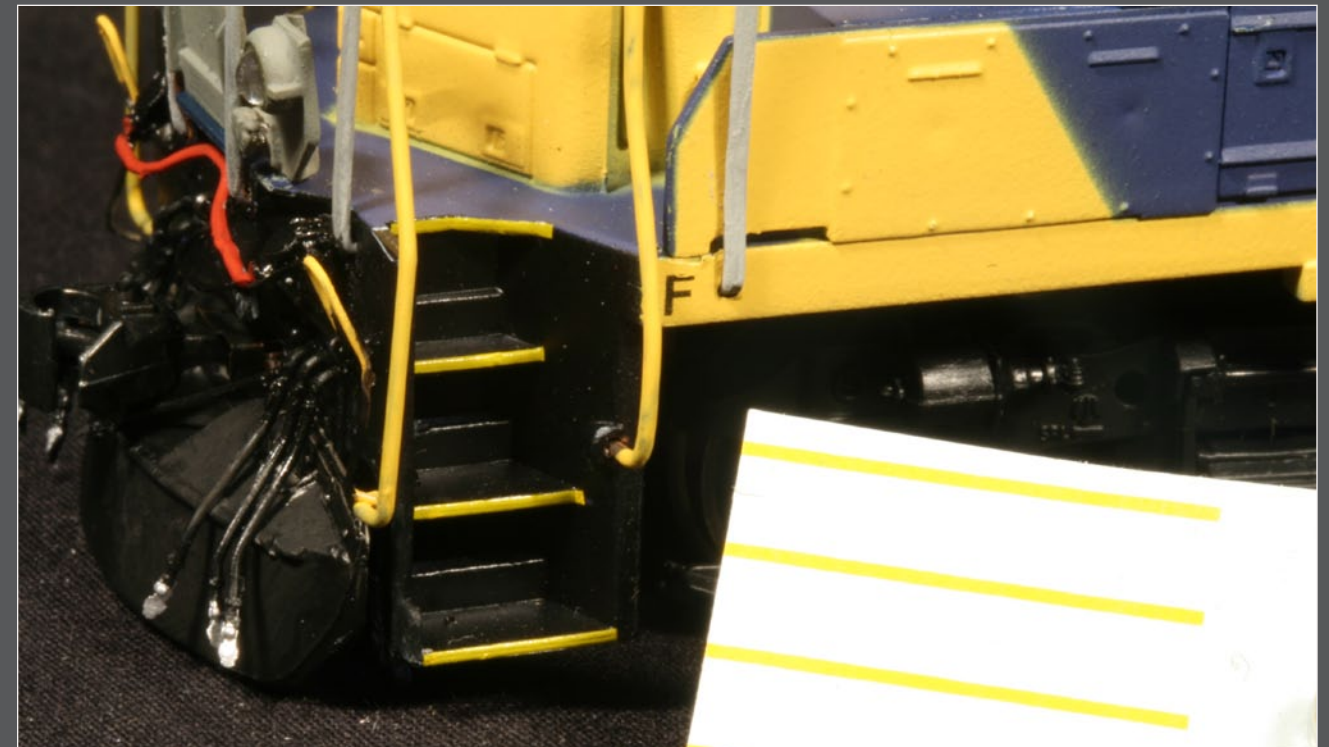
Figure 42: One thing that can really transform the appearance of a locomotive is coloring the step edges. Step edges are generally painted bright colors for visibility and can be easily decaled using 2" striping.
