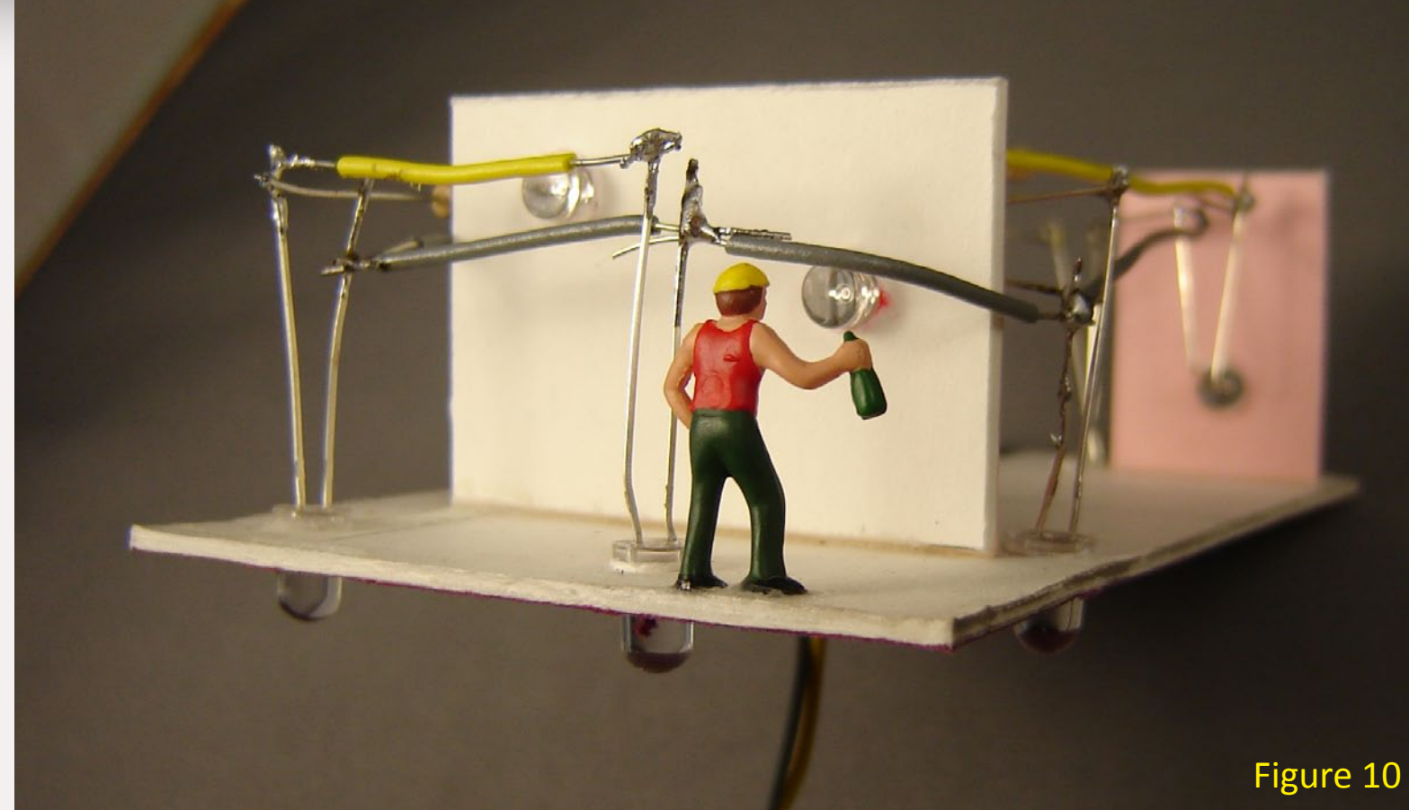
Figure 10: The figure that casts the 2nd floor shadow. The yellow LED is right in front of his face.
