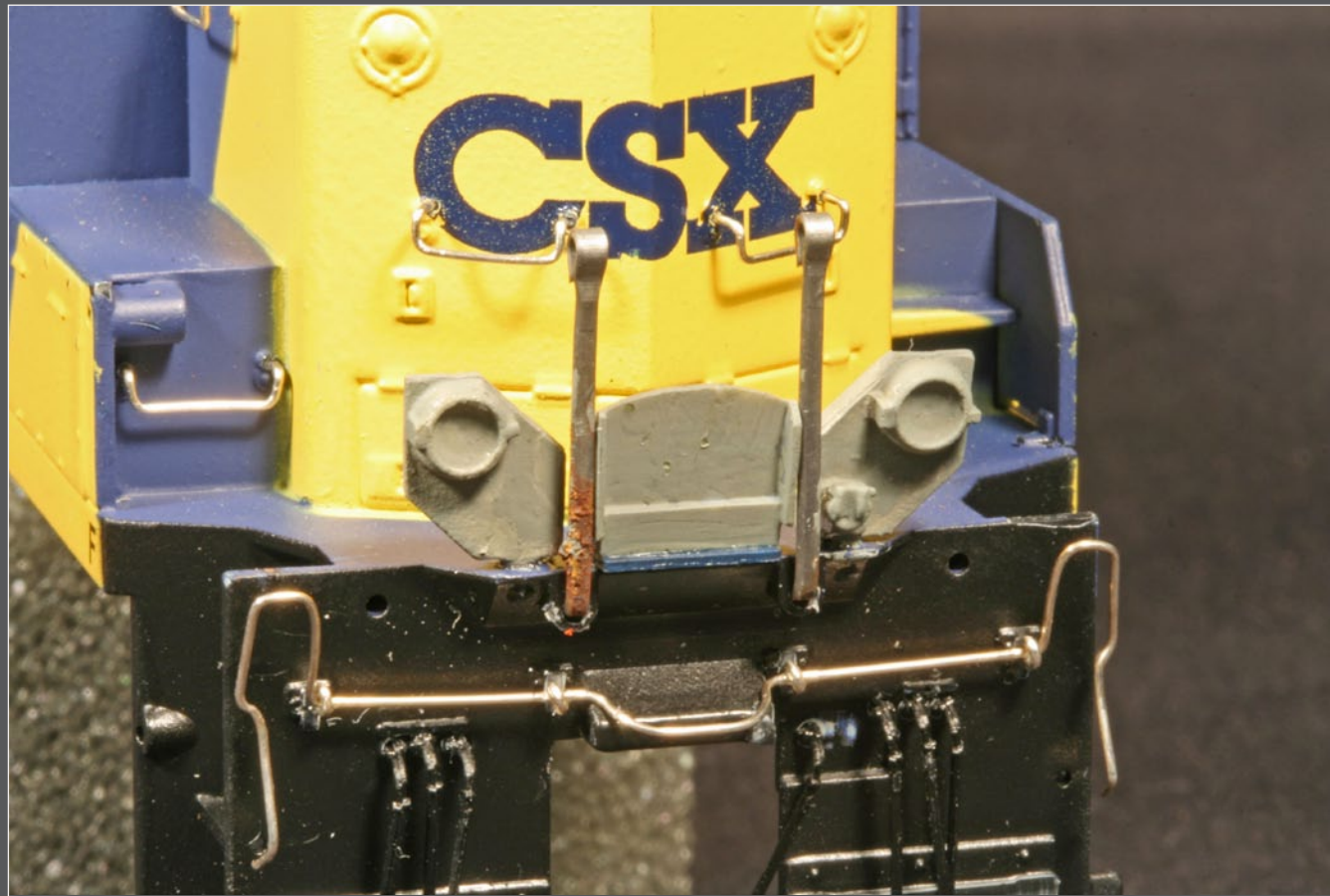
Figure 35: Many older locomotives have been retrofitted with ditch lights. Castings are available in several different styles, many with the capability of lighting.
