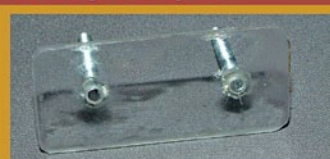
Figure 2: The plastic base for the cleaning pad with threaded rods flush with the sheet.
