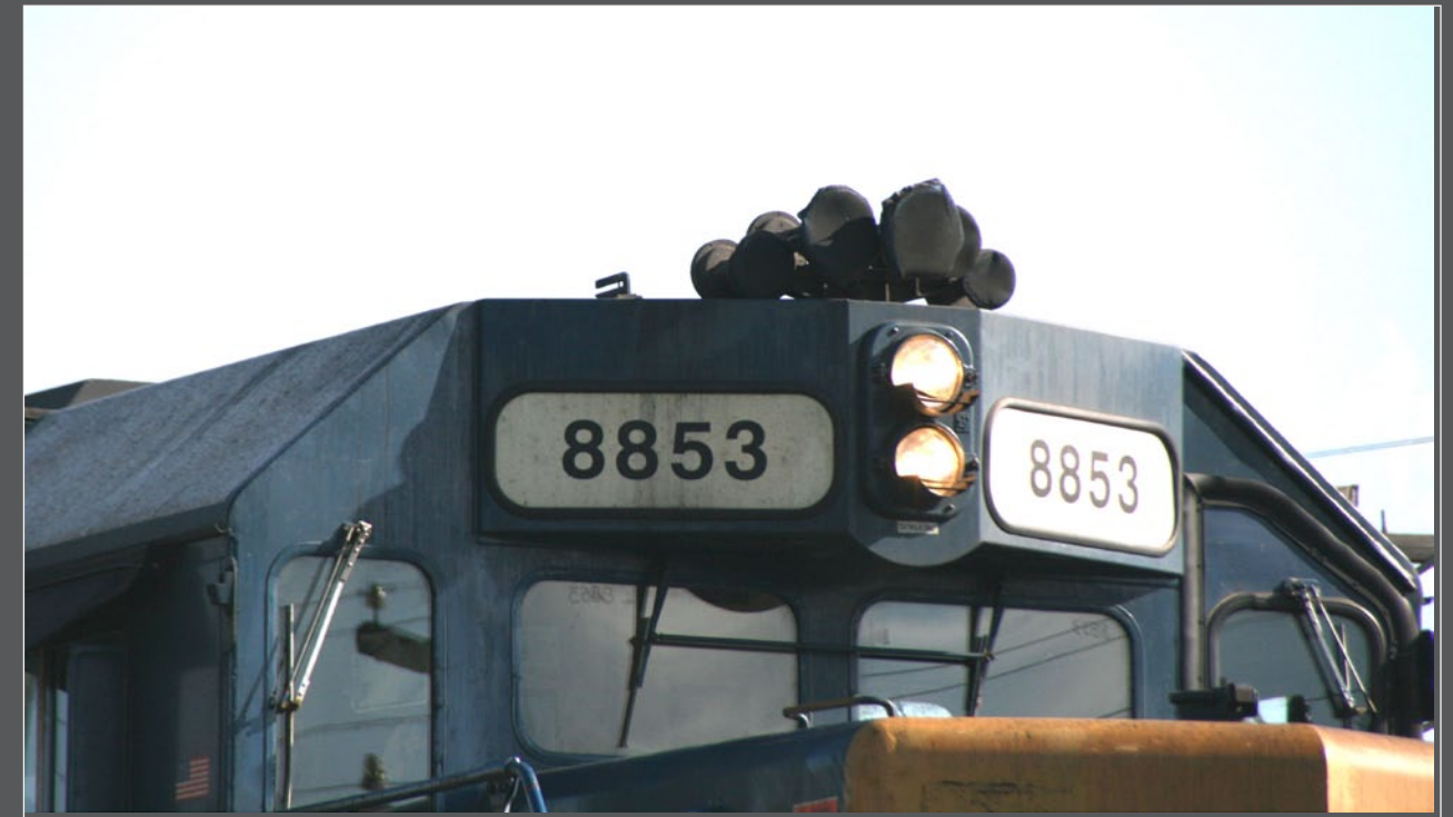
Figure 27: Roof details are often a mystery, as we often view the prototype at ground level. Several common details applied to cab roofs are a horn, radio antenna, and end-of-train antenna.
