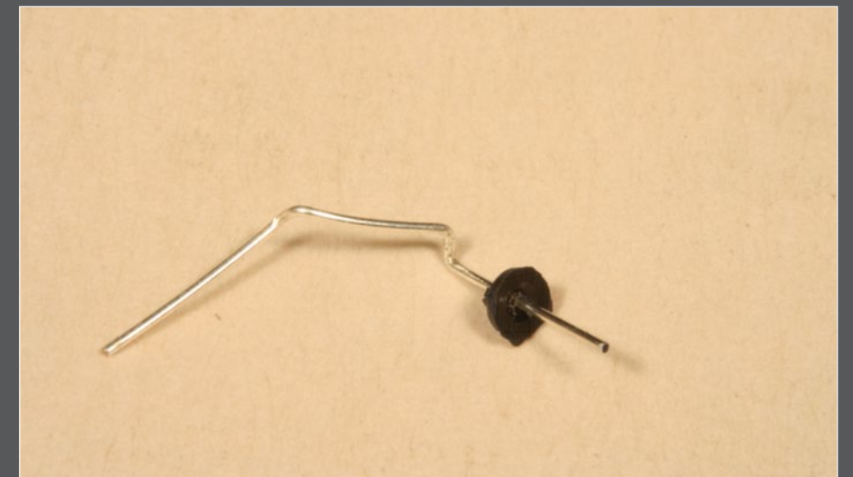
Figure 31: While castings for a 'whip style antenna' are available most only include the base. The actual whip can be added using fine wire or even one leg of a grabiron.
