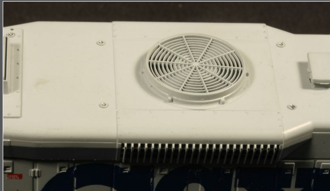
Figure 11: Some locomotive models were available in either dynamic or non-dynamic brake versions and can be easily identified by the large “blister” of the dynamic brake fan.
