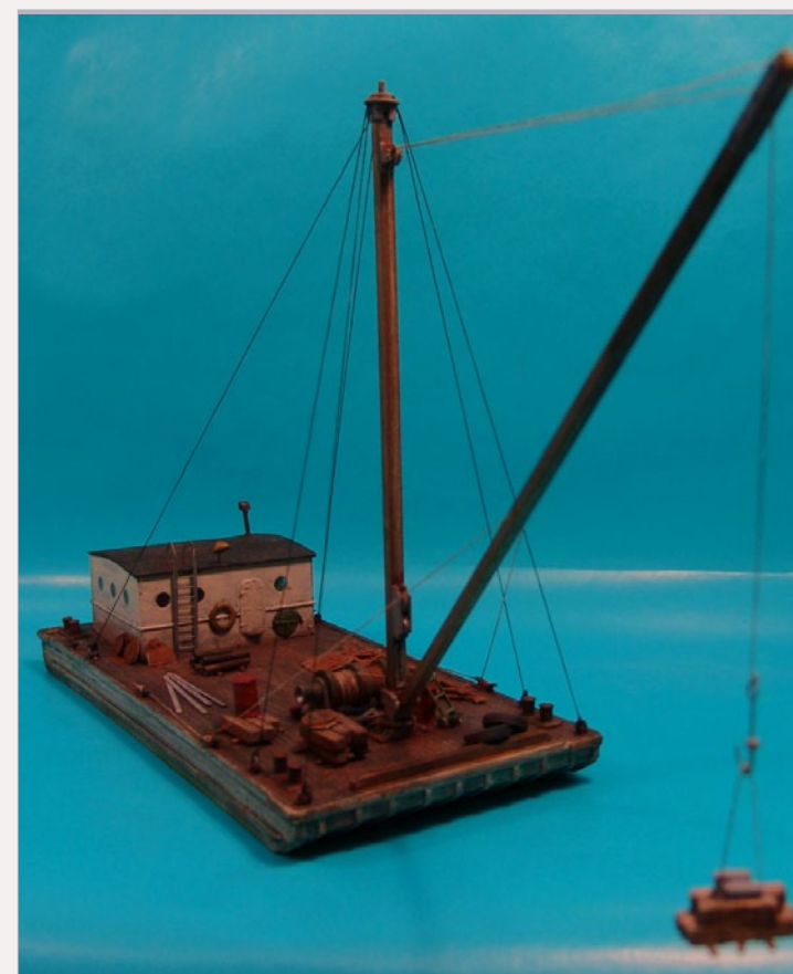
FIGURE 16: Seaport Model Works ( www.seaportmodelworks.com ) has a solid resin kit for an HO scale 57-foot flat barge. Components for the waterline model include a solid resin hull, photo-etched brass cabin and ladder, a cast resin cabin roof plus an assortment of special metal castings for the mast and boom assembly. The finished barge measures 8-inches long by 3.75-inches wide.
