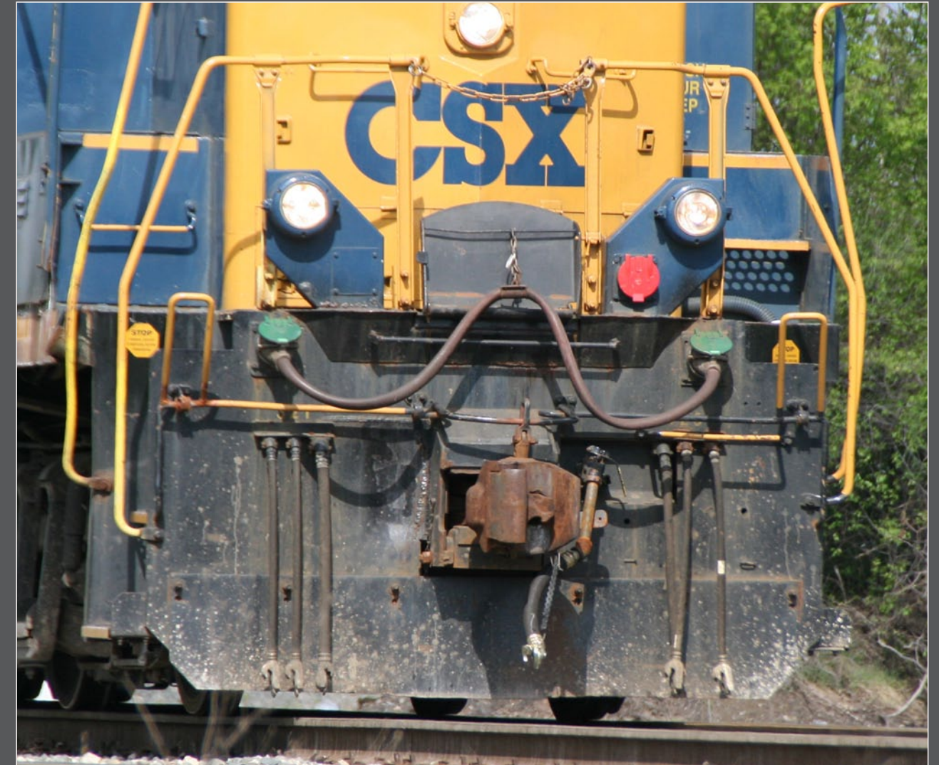
Figure 33: Illustrated in this photo are the ditch lights and drop step (visible above the locomotive walkway), and MU cable (the large cable looping across the top of the pilot).
