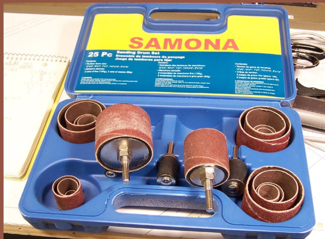
Figure 26: A simple drum sanding kit which made enlarging the holes go smoothly. Now why didn't I think of that? I have so many tools in my arsenal, but (until now) not this one!
