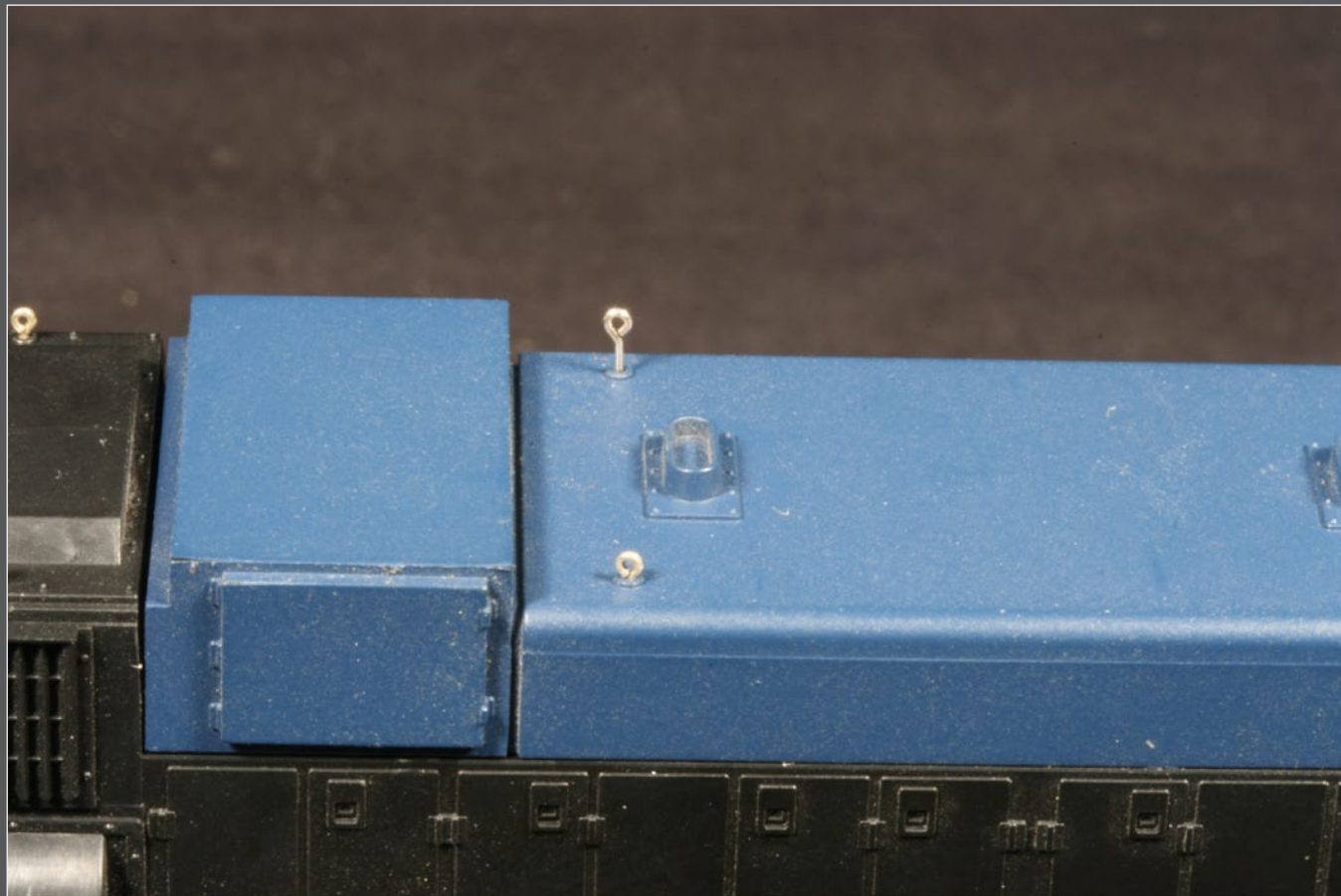
Figure 12: Prior to applying cement test fit each eyebolt to insure it is not too long. If it is, shorten it with wire cutters.
