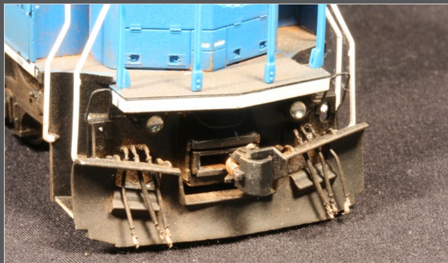
Figure 22: MU hoses are available in ‘clusters’ or as individual hoses, allowing the modeler to recreate any combination.
