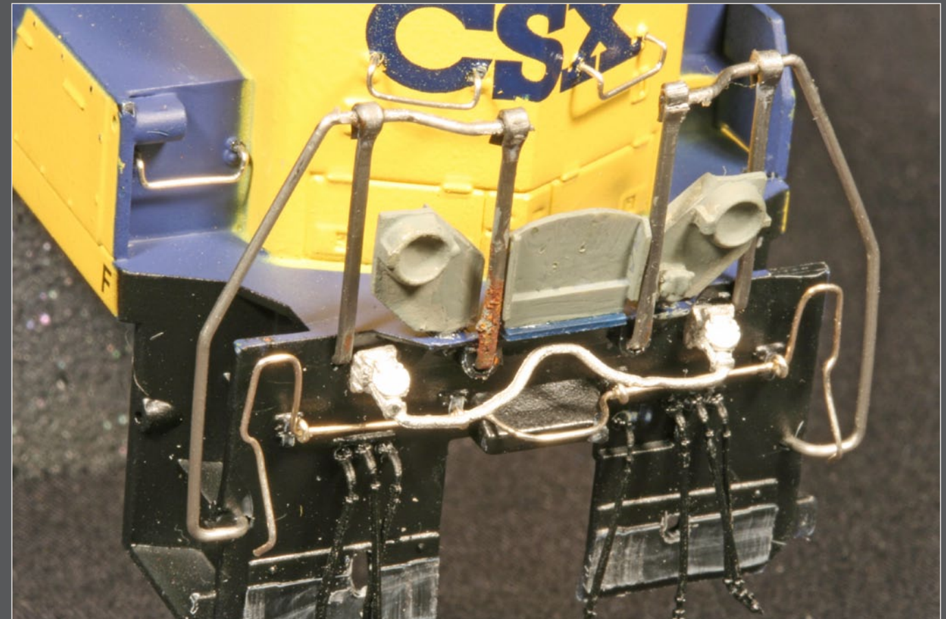
Figure 36: Metal MU cable castings will allow bending, giving the look of a cable tethered to the pilot of the locomotive.
