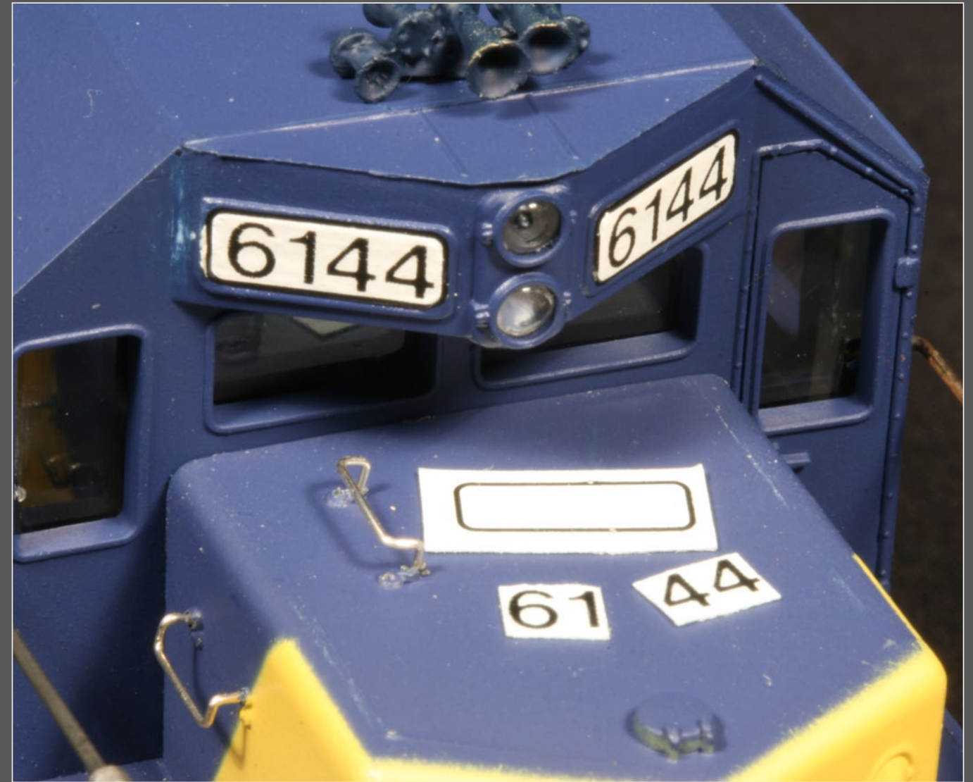
Figure 38: One detail modelers often overlook is the numberboards. The numberboard background can be either painted or decalled white or black, then number decals can be applied.
